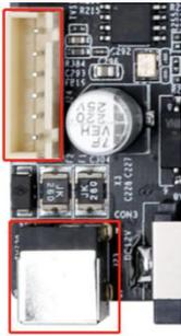
Interface definition as below list, user can apply power board input power supply, interface have 6PIN and 2.54mm pin distance.
