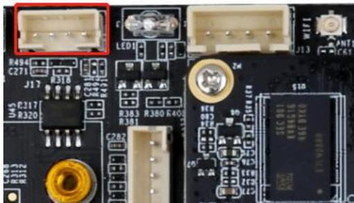
Motherboard provides a 485 serial port which can support mainstream serial ports devices. The voltage for 485 serial ports is 3.3V, if device connected require higher voltage, there must be an isolate circuit or level-shift circuit added, otherwise board and device might get burnout.
